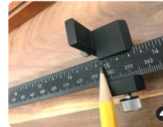
4 Adjust end stop at desired distance from the marked bushing
