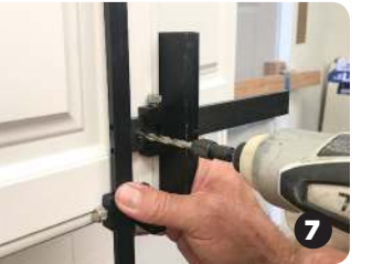
7 Reverse tool position onto opposite door and drill
