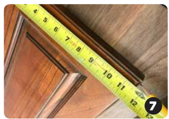
7 Measure height of drawer use half that number for center
