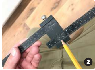
2 Align each ruler at the 5" mark to extend the length of ruler to 17"
