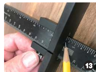
Adjust Large Stop to 1 3/8" to match the measurement from side edge
