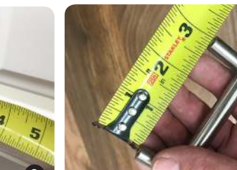
4 Measure hole centers of your hardware
