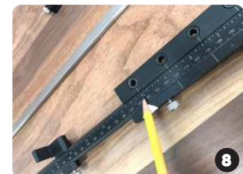
Set end stop at desired distance from center line of bushing
