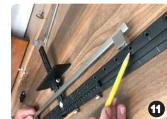
Match top hole on hardware to matching hole on extension
