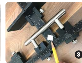
tighten sliding bushings into position cover the center bushing with tape
