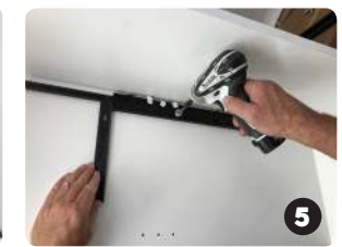
Remove Large Stop and press thumb screws against back panel then drill
