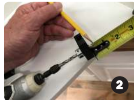
Set stop collar to drill depth
