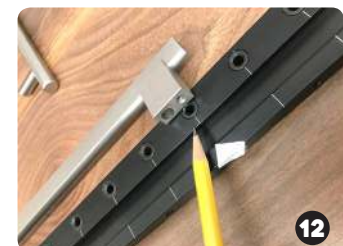
Mark hole location with tape
