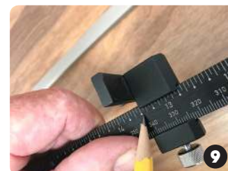
Set the sliding end stop 3 1/2" out on the era from bottom hole
