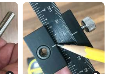
5 Transfer your hardware measurement to the sliding drill bushing and tighten
