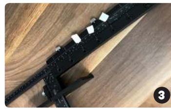
Mark your holes with tape for reference
