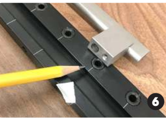
6 Now mark the other hole with tape
