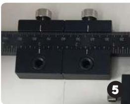
Setting two blocks together produce industry standard 32mm spacing
