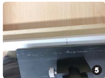
Line up notch on center of Large Stop with center mark at top of drawer then push tool flush against drawer face.
