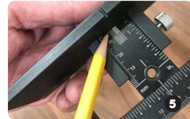
5 Match Large Stop to your side measurement and tighten
