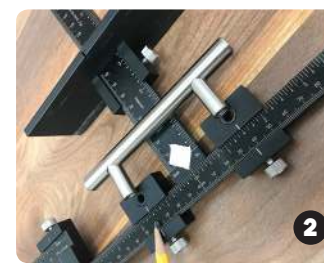
slide two drill bushings onto the tp-1934 Using the same measurements
