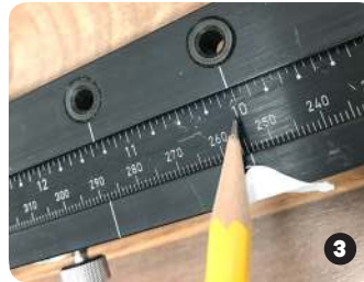
3 Mark selected drill bushing with tape on extension (included in TP-2312, TP-1935)
