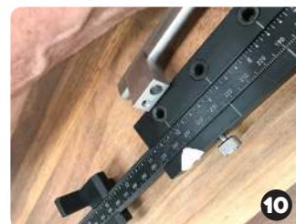
Match the bottom hole on hardware to bottom hole on extension and mark with tape
