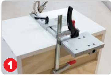
1 Clamp jig in desired light location
