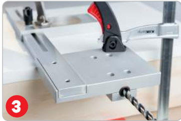
3 Leave clamps in place, drill wire hole until drill bit reaches light hole
