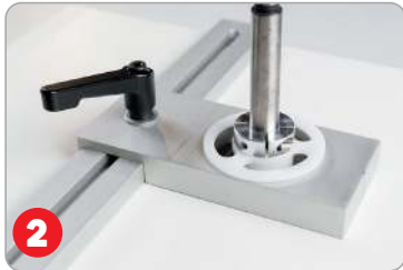
2 Drill light hole to desired depth using the adjustable stop
