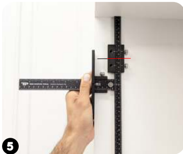
5 Place two Drill Guides side by side to achieve 32mm spacing. Position tool with Large Stop and T-square firmly against cabinet surface. Adjust Drill Guide centers to previous mark and tighten. Drill first set of hinge plate holes.
