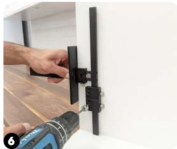
6 Flip tool to bottom of cabinet, position tool with Large Stop and T-Square firmly against cabinet surface, and drill second set of holes.
