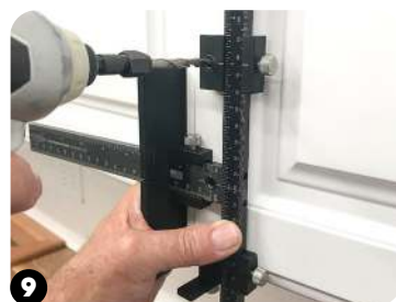
9 Drill through Drill Guide for top hole.
