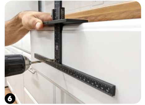
6 Hold securely and drill hole using fixed center drill bushing ( Large Stop reversed for stability).
