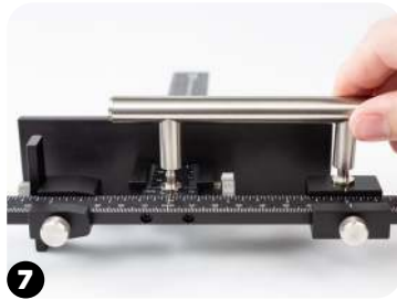
7 Set hardware onto spacing pins and press down until fully seated. Tighten thumb screws to set spacing.
