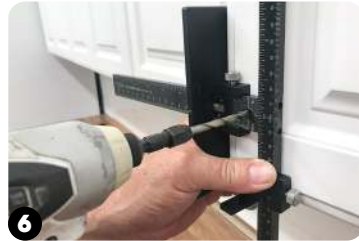
6 Position tool with stops as shown and drill hole through drill bushing.
