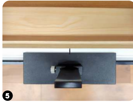
5 Line up notch on center of Large Stop with center mark at top of drawer then push tool flush against drawer face.
