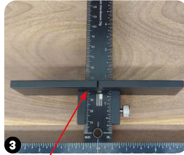
3 Set Large Stop to 37mm (industry standard).
