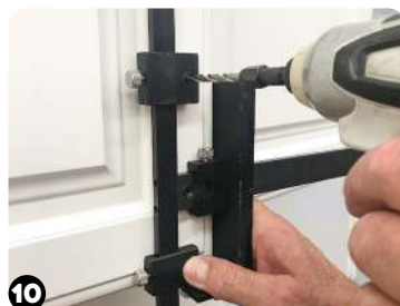
10 Flip tool to its reverse side, place on opposite door and repeat.
