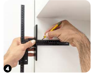
4 Place Large Stop edge against cabinet face and use as a square to draw a line at mark from Step 1.
